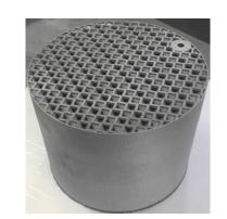
**ORNL** prints intensified devices with heat exchanger integrated into pack
